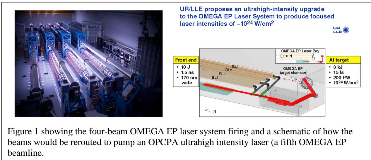
Figure 1 showing the four-beam OMEGA EP laser system firing and a schematic of how the beams would be rerouted to pump an OPCPA ultrahigh intensity laser (a fifth OMEGA EP beamline).
