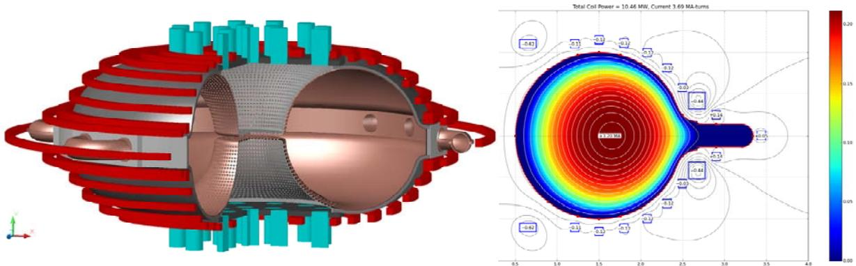
**Figure 1** On the left: Engineering conceptual design, the teal cylinders are cryo-pumps. All surfaces in the vacuum will be covered with an insulating ceramic. On the right: Physics conceptual design, the contours are beta engineering =  $2\mu_0 p/B_{wall}^2$  where  $B_{wall} = \mu_0 I/2\pi a$ . Table 1 gives parameters of this PoP experiment.
