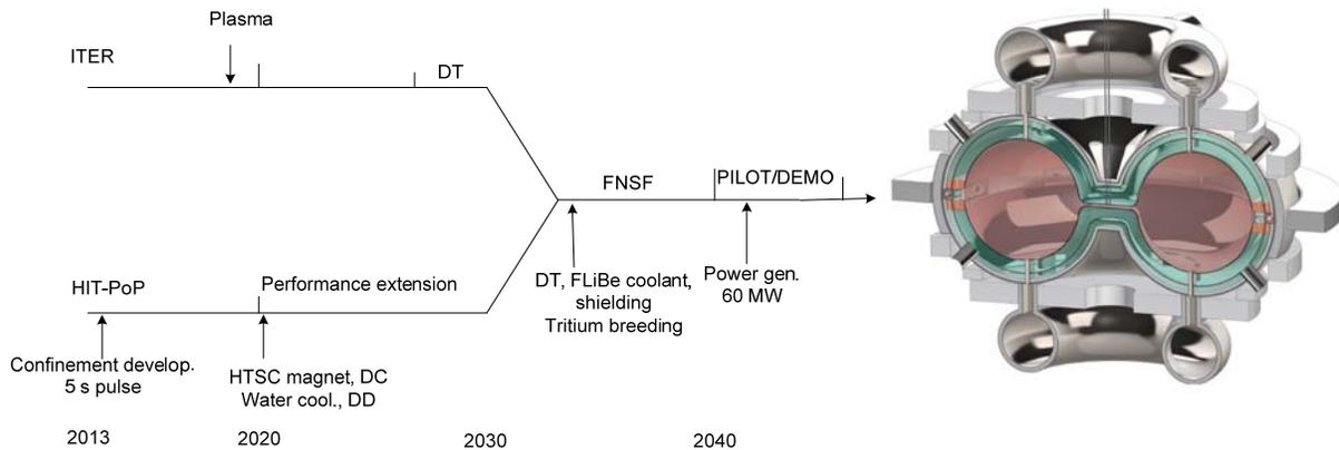
**Figure 2. Time line to fusion power generation. HIT-PX, FNSF, and Pilot/DEMO are the same facility with the plasma the size of HIT-PoP. The FNSF has the parameters of Pilot/DEMO in Table 1. The drawing on the right is of the 1 GW reactor<sup>2</sup> with parameters given in Table 1. The entire first wall is the limiter.**
