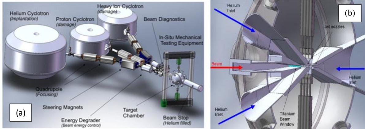
Figure 1. Triple cyclotron beam line for protons, helium, and heavy ions (a). Target chamber (b).
