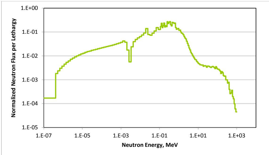
**Project X Energy Station Spallation Neutron Spectrum with 1 GeV Incident Proton Beam (After Wootan and Asner 2012).**
