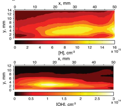
Figure 2b - 2D, absolute distributions of H and OH in ns pulse, surface ionization wave plasmas sustained over liquid water in Ar buffer, measured by LIF / TALIF.
