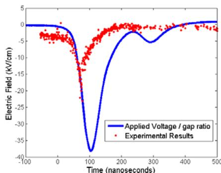
Figure 2a - Time-resolved electric field in a ns pulsed H<sub>2</sub> plasma measured by ps CARS / 4-wave mixing with 0.2 ns resolution.
