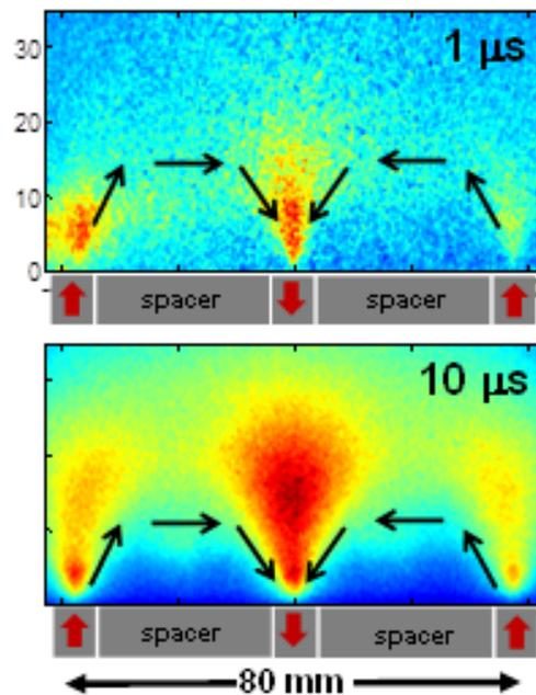
Figure 1 – LIF measurements of the evolution of He excited states above a magnetic cusp.
