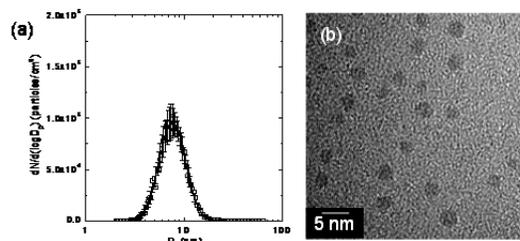
Figure 6b (left) On line aerosol mobility measurements and (right) carbon nanoparticles nucleated from ethanol vapor in an atmospheric pressure microplasma.
