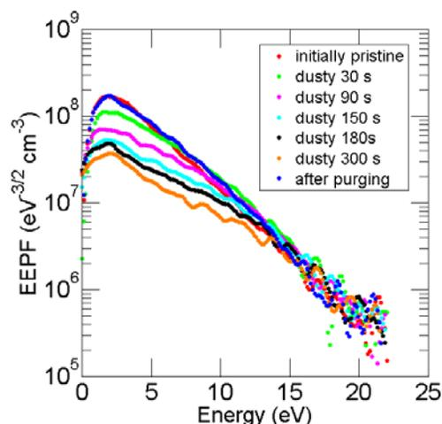
Figure 6a – Electron probability distributions in an 80 mTorr Ar/SiH<sub>4</sub> plasma with a growing inventory of nucleating nanoparticles.
