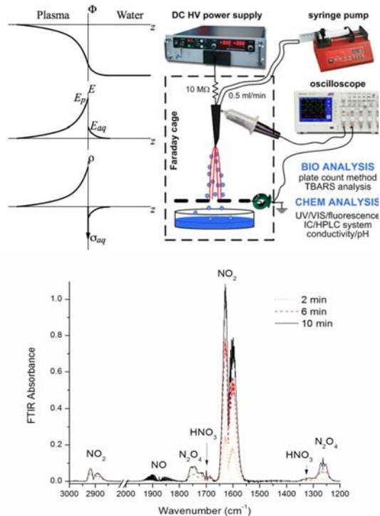
Figure 3 - (top left) Anticipated charge densities, electric fields, and potentials near the plasma-water interface. (top right) Experimental system investigating plasma-water droplet interactions using electrospray and pulsed/transient streamers and sparks. (bottom) FTIR spectrum of gas phase species from air plasma.
