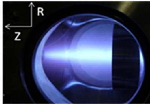
Figure 7 – Magnetized LTP in Xe that for control of  $f(\vec{r}, \vec{v}, t)$  which separates “hot” electrons from cold electrons with a magnetic filter. Anomalous transport due to instabilities may affect the efficiency of the magnetic filter.
