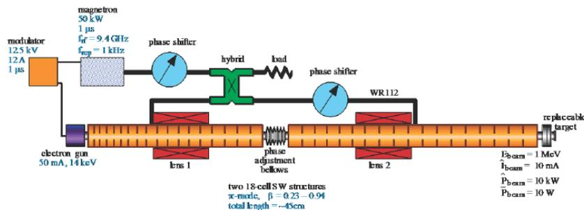
Figure 7. X-band compact LINAC and components developed at SLAC as a compact x-ray source. See text for details.
